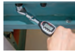
It can be used with the head turned over
