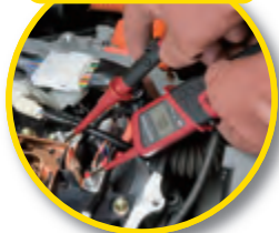
Voltage measurement prior to work is specified in the manufacturer manual.
